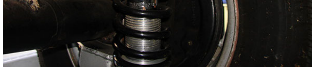
The upper chassis mount uses the old shock absorber mounting holes.
