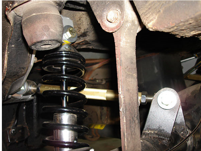
Stock bump stops and rebound straps can be left unchanged. (For added safety, when you weld the mounting tabs onto your axle you may want to weld a simple reinforcement strap or two between them to reduce the likelihood of fatigue cracking in the welds.)
