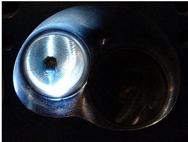
Here is a closer look at the combustion chamber and intake port...
