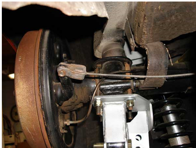
The Classic Conversions 4-link provides a full range of suspension travel without binding. (The lower end of the shock absorber has been disconnected for this demonstration photo.)
