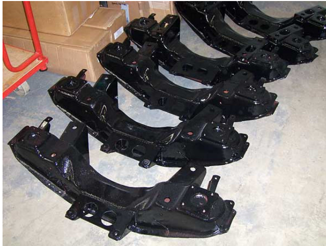
MGB front crossmembers with modifications for power steering.
