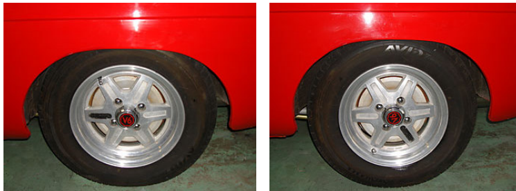
These two photos show the suspension's lowest and highest static height settings.
