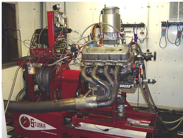
Awesome Engines makes sure all their engines produce whatever they're supposed to before shipping. Here's a Big Block Chevy on the dynamometer. Take a look at the dyno print-out below.
